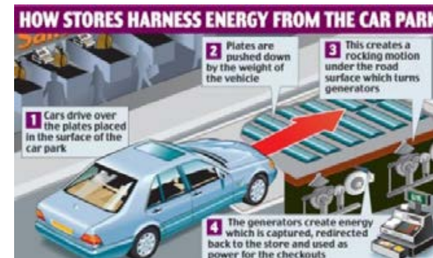
Electrokinetic road ramps generate power from the force of a crossing automobile. This technology is ideal for parking structure entrances.
