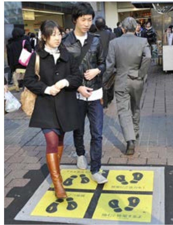
Piezoelectric flooring generates electricity from pedestrian traffic. Additional locations include stairs and playgrounds.
